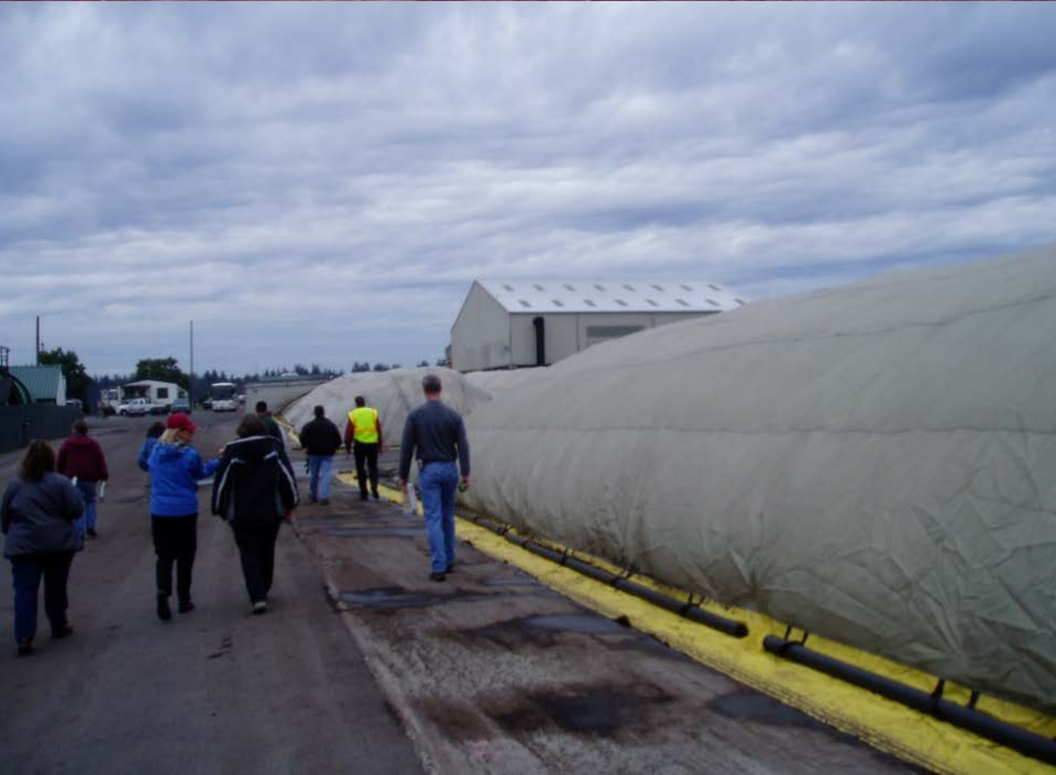
Aeration trenches under the Gore covers. Three phase composting. 2 phases under the covers + 1 curing phase.
